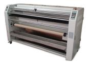
Simple to operate, the Starlam 64" roll to roll laminator applies a smooth, even layer of ClearShield laminate over a wide variety of substrates.
