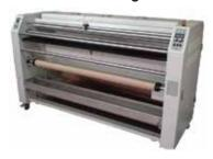
The StarLam 1600R Roll-to-Roll Liquid Laminator is easy to operate and applies a smooth, even layer of ClearShield Liquid Coatings over a variety of substrates. The StarLam is ideal for large volume production environments and store-front shops alike. For more information on the StarLam 1600R Roll-to-Roll laminator, visit us online at www.marabu-northamerica.com
